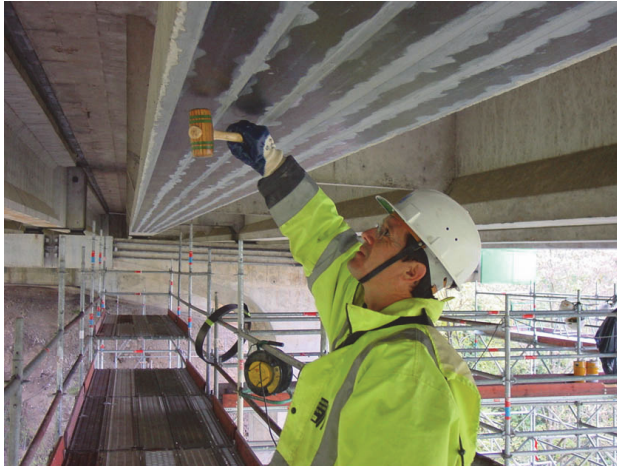
Fig. 1. Inspection with acoustic sounding (hammer tapping).
