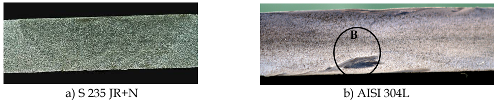
Fig. 31. Macroscopic aspect of welded joints
