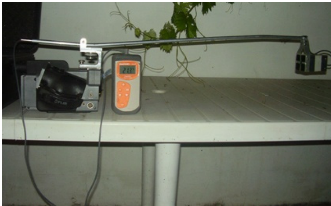
Fig. 4. Setting of field observations. The camera was attached in a permanent position at one end of a special "antenna", and the blackbody was situated at the other end, with the hole facing the camera. The distance between the lens and the blackbody was 80 cm. At the right-hand side of the picture can be seen the wire that connected a temperature probe that was inserted into the rear of the blackbody to the digital thermometer, which is displayed in front of the camera only for this photograph. During experimental measurements this thermometer was carried in a small bag, and the digital blackbody temperature was recorded manually for each thermogram.
